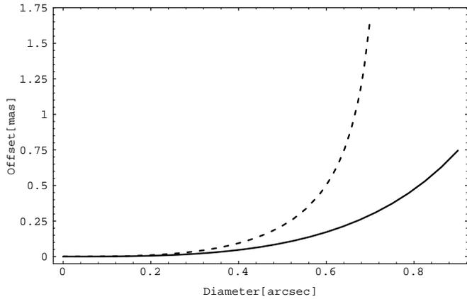
**Fig. 9.** Theoretical difference between the observed position and the photocentre versus apparent diameter. The graphs correspond to a spherical object of uniform brightness viewed with a solar phase angle  $\alpha = 20^\circ$ . Solid curve: positions derived from the first harmonic only (NDAC). Dotted curve: positions derived from a weighted mean of the harmonics (FAST) — this method is in practice limited to objects smaller than 0.7 arcsec
