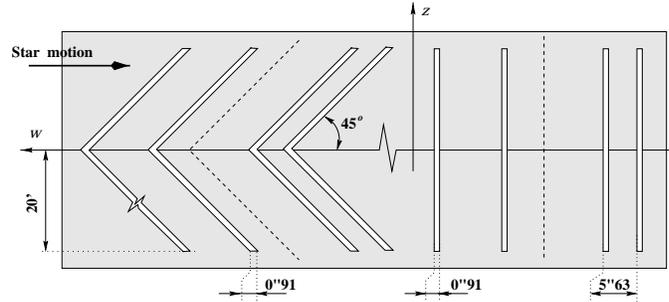
**Fig. 4.** Schematic view of the star mapper slits system. All slits have the same width in the direction of the  $w$  axis. The inclined and vertical slits are spaced, in the direction of a star’s motion, at distance ratios 2:3:1 of the step  $s = 5.63$  arcsec. The ‘fiducial lines’, which can be thought as the centres of gravity of the four slits in each group, are shown as dashed lines
