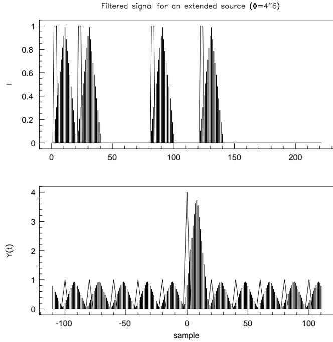
**Fig. 5.** Simplified profile for the photon count of a point-like source and a circular extended object of apparent diameter  $\phi = 4.6$  arcsec (top). Both intensities are normalised to unity. This signal is folded by a digitalised filter (bottom); the position and amplitude are then derived from the Q integer detection filter [-1,-1,-1,0,+1,+1,+1]
