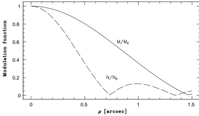
**Fig. 8.** Modulation function for the first two harmonics of a uniformly bright disc as a function of the apparent diameter  $\rho$
