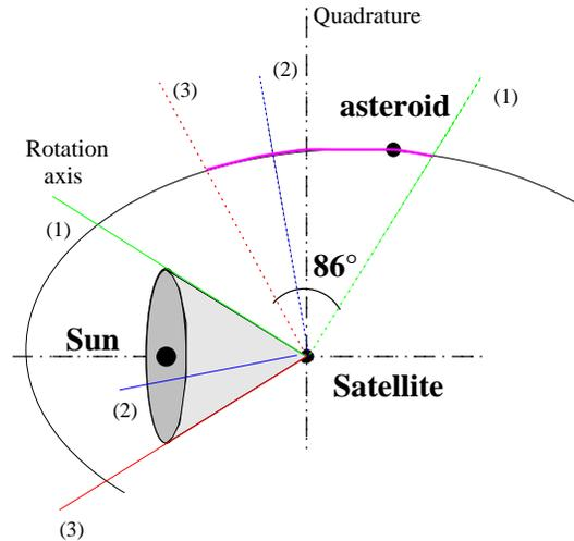
**Fig. 1.** Schematic view of the Hipparcos satellite scanning procedure (or scanning law). The rotation axis describes a cone around the direction of the Sun. The observations of solar system objects, at right angle to the rotation axis, were made around the quadratures, bounded by positions (1) and (3)
