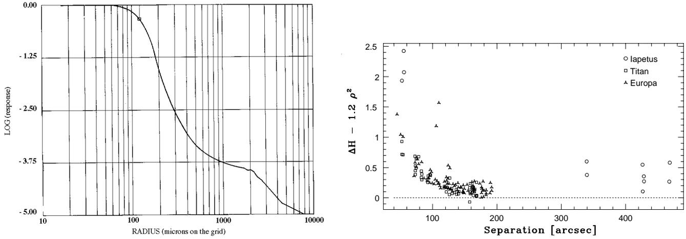
**Fig. 10.** Attenuation profile. Left: average profile from on-ground calibration ( $8 \mu\text{m} = 1.208 \text{ arcsec}$ ). The actual in-flight profile is unknown between 100 and 500 arcsec. Right: magnitude difference  $\Delta H$  corrected for bias due to the modulation as a function of the separation to the major planet
