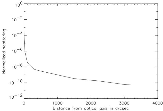
**Fig. 1.** Measured normalized scattered light distribution of the SUMER telescope as a function of focal plane distance (from Saha & Leviton 1993).
