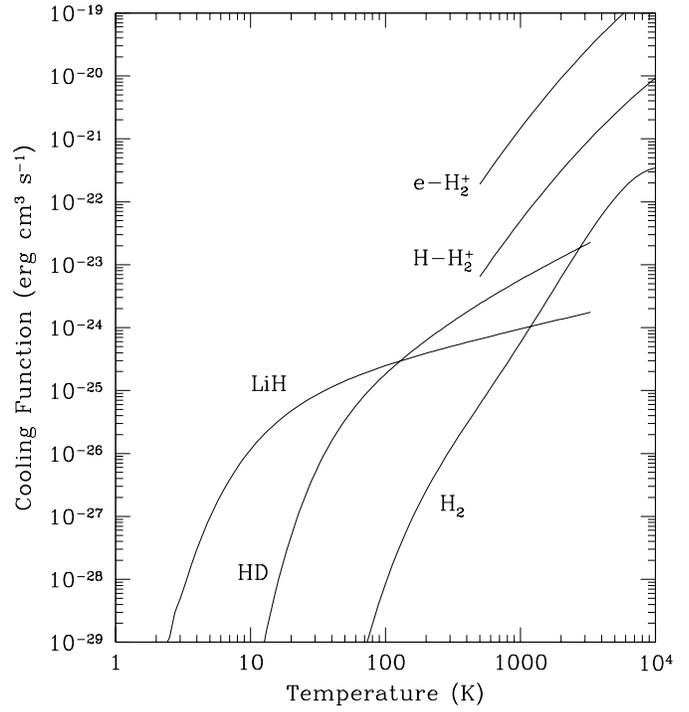
**Fig. A2.** Cooling function per molecule of H<sub>2</sub>, HD, LiH and H<sub>2</sub><sup>+</sup> in the low density limit ( $n(\text{H}) \lesssim 10^2 \text{ cm}^{-3}$ ).
