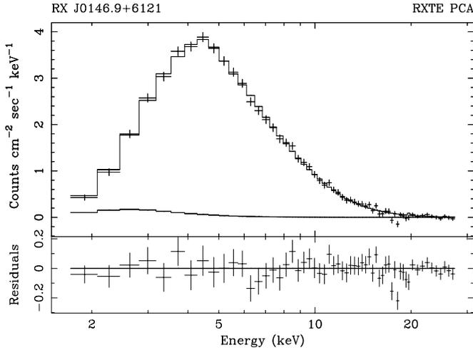
**Fig. 4.** Average X-ray spectrum over the complete RXTE observation. The best fit power-law model with high-energy cutoff (see text) is plotted as upper histogram and the residuals are shown in the lower panel. The contribution of 4U 0142+61 is indicated by the lower histogram
