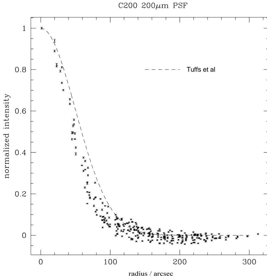
**Fig. 3.** Mapping measurements of the point source NGC 7027 taken in the ISOPHOT  $200\mu\text{m}$  filter. The markers denote the relative intensity against radial distance from the central position. The dashed line shows the gaussian approximation (FWHM  $\simeq 117''$ ) used by the ISOPHOT instrument team to describe the  $200\mu\text{m}$  beam (Tuffs et al (1996)).
