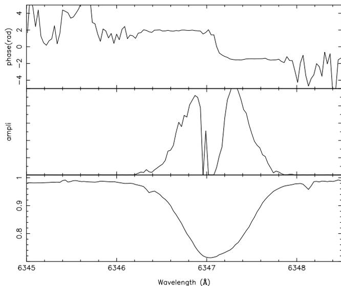
**Fig. 8.** Amplitude and phase diagram of  $f_1$  of  $\theta$  Tuc, as derived from the periodogram shown in Fig. 7. In the bottom panel we show the mean profile of the Si II 6347 Å line, in the middle the amplitude distribution is given, and in the top panel we show the phase diagram with the ordinate in radians.
