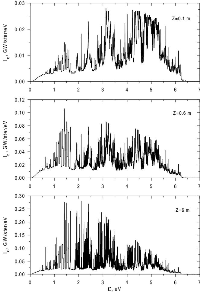
**Fig. 6.** The theoretical spectra at altitude 40 km for  $R = 0.42$  m,  $V = 20$  km s<sup>-1</sup>, and different lengths  $Z$  of the luminous volume.
