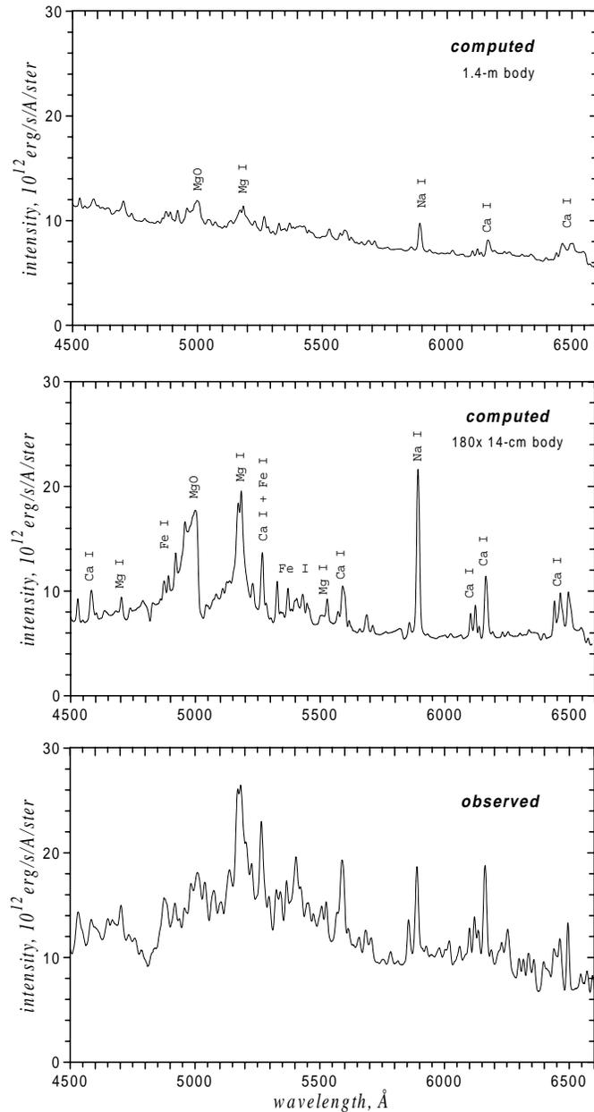
**Fig. 10.** Comparison of the observed spectrum at altitude 24.5 km and the modeled spectra for 180 independent fragments with radii 0.14 m and one single body with radius 1.4 m at altitude 25 km. The velocity is  $15 \text{ km s}^{-1}$ .
