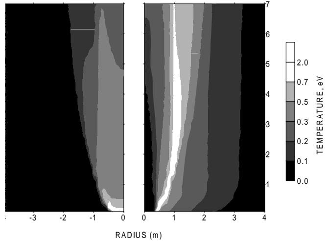
**Fig. 2.** Distribution of the brightness temperature in the panchromatic passband (left side) and the real temperature distribution (right side) computed in the framework of the ablation model for the body radius 0.42 m, velocity  $20\text{ km s}^{-1}$ , and altitude 40 km.
