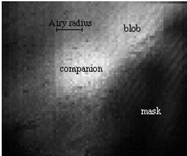
**Fig. 2.** Laboratory simulation of stellar companion detection with the dark speckle method. The artificial companion, 966 times fainter than the star, is at the center of the dark map, emerging from the halo. A coronagraphic mask, which hides the star's central peak is visible in the lower right corner. The blob seen in the upper right part of the field is a "static speckle" caused by permanent aberrations and removable with a reference star.
