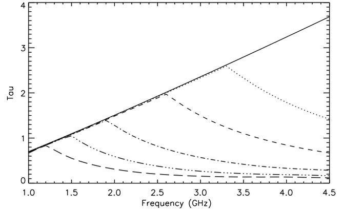
**Fig. 3.** The optical thickness of the 1-4.5 GHz plasma emission on harmonic frequency during the evaporation shock propagation at 0 s (full line), at 4.91 s (dotted line), at 8.44 s (dashed line), at 11.41 s (dot and dashed line), at 14.07 s (dot-dot-dot and dashed line), and at 16.49 s (long dashed line).
