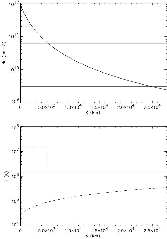
**Fig. 1.** The initial density and temperature profiles of the flare atmosphere (full lines). The dashed line expresses the equilibrium temperature profile. The evaporation shock is initiated by a temperature jump (dotted line).
