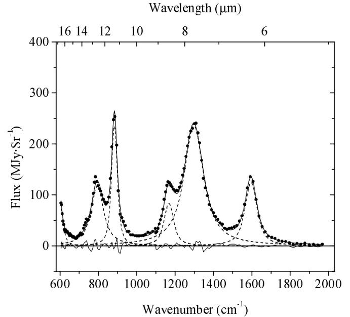
**Fig. 4.** The main bands fitted by Voigt profiles (Lorentz profiles convolved by the instrument resolution, see Sect. 3.2.1 for details). The symbols are the same as in Fig. 1. The minor bands and the linear baseline of Fig. 1 have been subtracted from the data.
