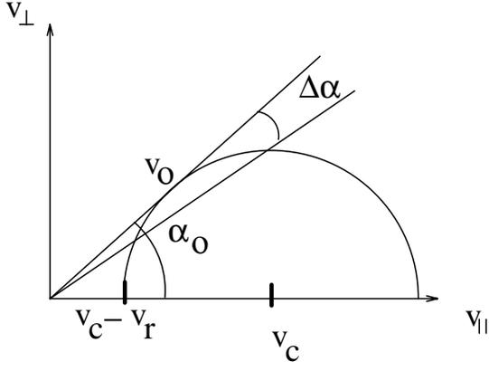
**Fig. 1.** The resonance circle is placed so it is just touching the edge of the loss cone. Here, the loss cone extends out to the line at angle  $\alpha_0$  to the  $v_{\parallel}$  axis. The  $\partial f/\partial p_{\perp}$  derivative is positive only in a region of angular width  $\Delta\alpha$ . For  $\alpha < \alpha_0 - \Delta\alpha$ , the distribution function (and all its derivatives) is zero.
