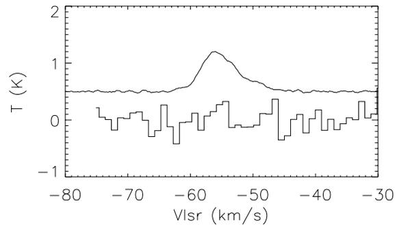
**Fig. 2.** The PIROG 8 observation of NGC7538 in the region of the O<sub>2</sub> 425 GHz line (lower curve) compared to the C<sup>18</sup>O (1–0) line (shifted by 0.5 K) as it would be if observed with the PIROG beam (constructed from the Onsala map). No O<sub>2</sub> line is detected.
