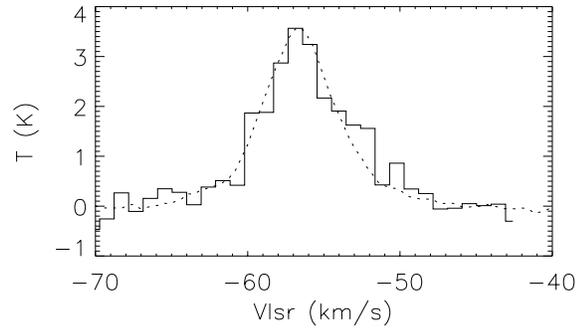
**Fig. 1.** The brightness temperature of the <sup>13</sup>CO (4–3) line of NGC7538 as observed with PIROG 8 scaled to agree with the expected line constructed from CSO observations (dotted line). The same scaling factor (6.7, equivalent to a beam efficiency of 0.15) between brightness temperature and antenna temperature was used for the O<sub>2</sub> observation.
