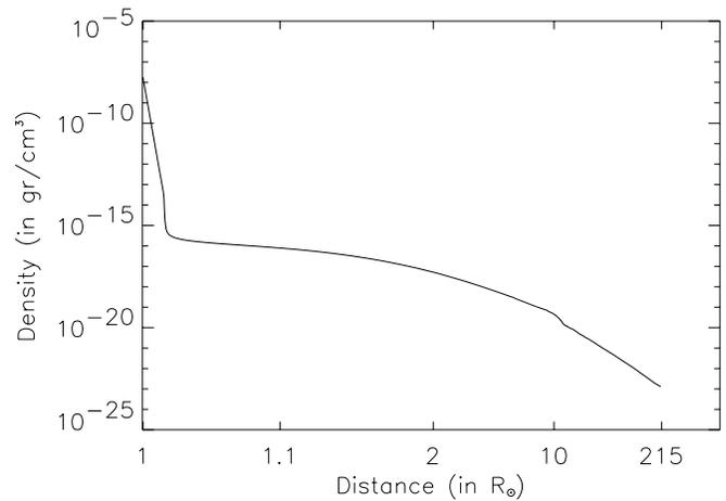
**Fig. 8.** The average profile (over 200000 timesteps) of the density  $\rho$  (in  $\text{gr cm}^{-3}$ ) as a function of heliocentric distance for the Alfvén wave pressure model.
