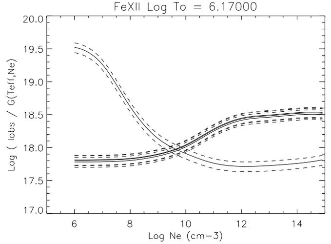
**Fig. 1.** Fe XII lines observed in CDS NIS 1 spectral range. The overlapping lines are the 346.8 Å, 352.1 Å and 364.4 Å transitions while the crossing one is the 338.2 Å transition. The  $\text{Log} T_{eff}$  is also shown at the top.
