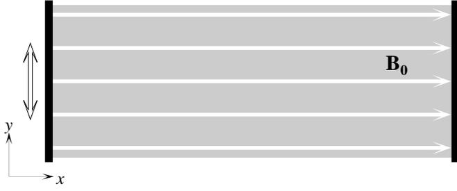
**Fig. 1.** Sketch of the cavity with one moving (*left*) and one fixed (*right*) boundary. The equilibrium pressure,  $p_0$ , density  $\rho_0$ , and magnetic field,  $\mathbf{B}_0$ , are homogeneous and constant in time.
