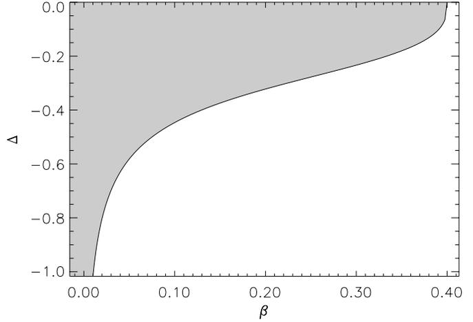
**Fig. 2.** The dependence of  $\Delta_c$  on  $\beta$ . Unique solutions exist in the shaded area. In the non-shaded area either unique or triple solutions exist depending on the value of  $R$ .
