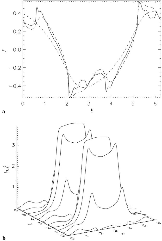
**Fig. 7a and b.** The solutions with shocks for  $\beta = 0.1$  and  $\Delta = 0.2$ . **a.**  $f$  vs  $\xi$  numerically calculated with  $N = 128$ . Note the progressive development of shocks as  $R$  is increased from 10 (short-dashed line) to 100 (long-dashed line) and 1000 (solid line). **b.** The time-evolution of the velocity field  $v(x, t)$  for  $R = 100$ .
