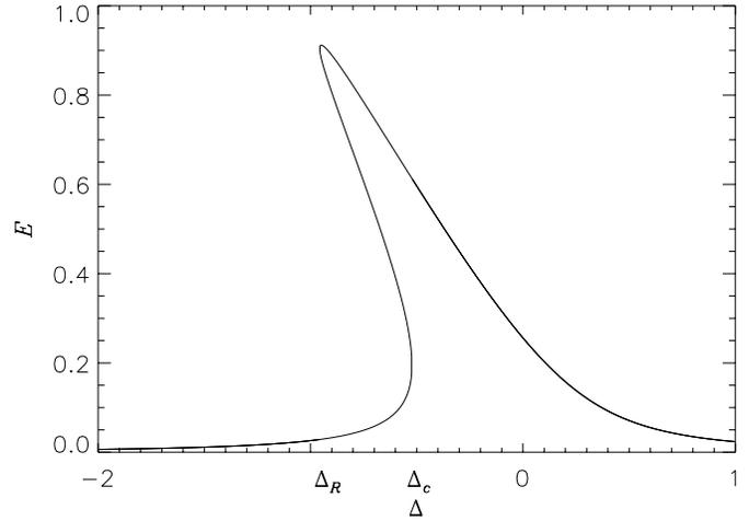
**Fig. 6.** Energy response of the cavity vs the normalized frequency mistuning at  $\beta = 0.1$  and  $R = 3$ . Note the similarity with the response curve of the Duffing oscillator.
