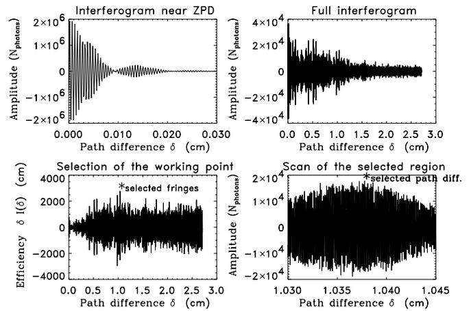
**Fig. 2.** **a** Interferogram near zero path difference. Intensity is scaled to the total number of photons collected within the filter; path difference  $\delta$  is in cm. **b** Full interferogram; beyond  $\delta \simeq 2$  cm, the interferogram is dominated by photon noise. **c** Efficiency function  $\delta \times I(\delta)$ ; the highest peak corresponds to the best working point. **d** Fine scanning of the fringe peak, and determination of the working path difference.
