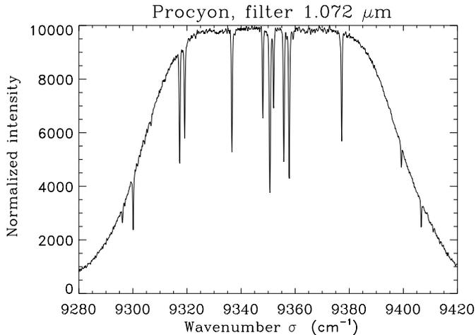
**Fig. 3.** Bandpass of the filter, selecting a dozen lines (mostly Si II lines) without any telluric contribution.
