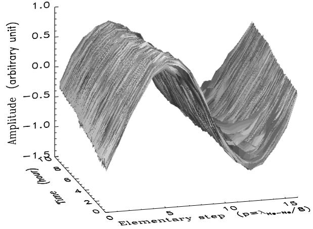
**Fig. 1.** Display of the fringe signal of a full night. The same fringe, corresponding to the optimized seismometric signal, is continuously scanned forward and backward along the entire night.
