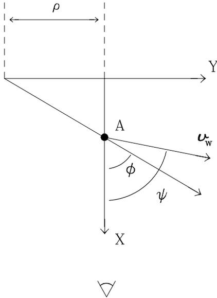
**Fig. 1.** Geometry adopted for calculation of the emission profiles from an elementary plasma volume located in A.
