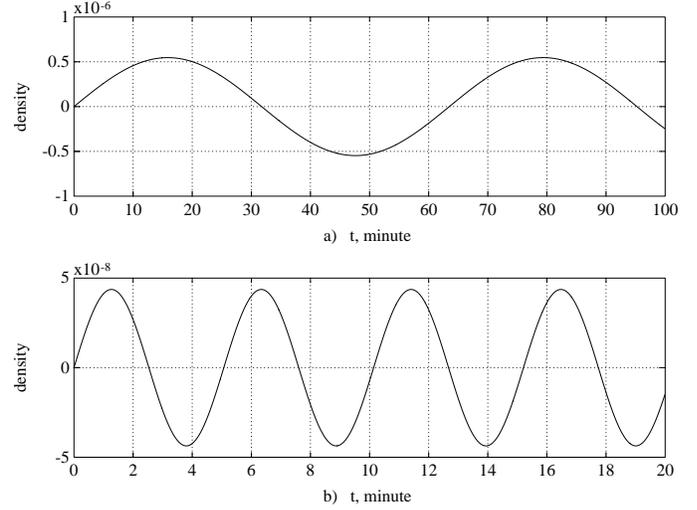
**Fig. 3a and b.** Short time interval for density perturbation in resonance case. **a**  $\beta = 2 \times 10^{10}$  and time is normalized on 1 minute. The period of fast magnetosonic waves is  $\sim 63$  minutes. **b**  $\beta = 3 \times 10^{12}$  and time is normalized on 1 minute. The period of fast magnetosonic waves is  $\sim 5$  min.
