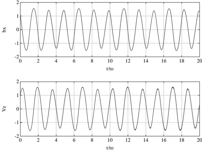
**Fig. 2.** Time evolution of the magnetic field and velocity perturbations in the case  $k_z = k_x = 1.2 \frac{\Omega_0}{2V_A} - 0.1k_y$ ,  $k_y \ll k_x$ . Here  $\beta = 2 \times 10^{10}$  and  $t_0 = 11$  yr.
