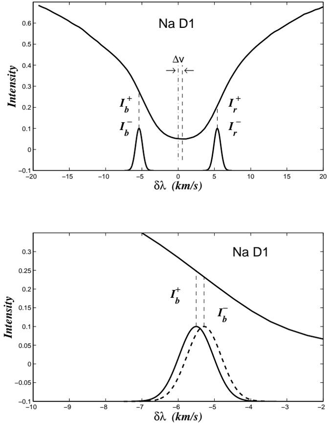
**Fig. 1.** Illustration of the operation modes *B* (top) and *C* (bottom) on GOLF instrument on one of the components of the Na doublet and for a given displacement  $\Delta V$  of the solar spectral line. The velocity position of the Blue and Red components corresponds to the center of the 1.2 Km/s region scanned by them. For *Mode C* only the region around the operating point is shown.
