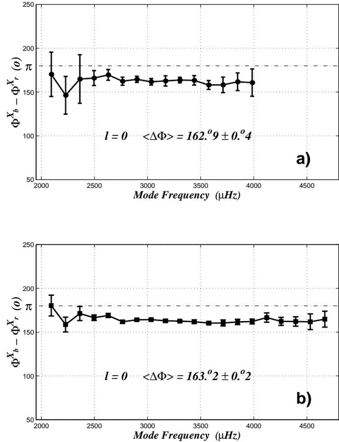
**Fig. 3a and b.** Phase difference between the  $\ell=0$   $p$ -modes measured through the GOLF blue ( $X_b$ ) and red wing ( $X_r$ ) signals, on simultaneous time series. In **a** the results obtained by direct comparison of the peaks' phase while in **b** results obtained from the bivariate analysis on the same series. In both cases,  $\langle \Delta\Phi \rangle$  is the weighted mean of the individual values for each mode.
