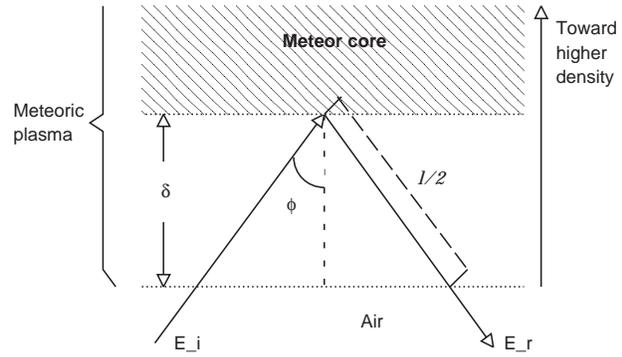
**Fig. 6.** Forward-scatter reflection geometry.
