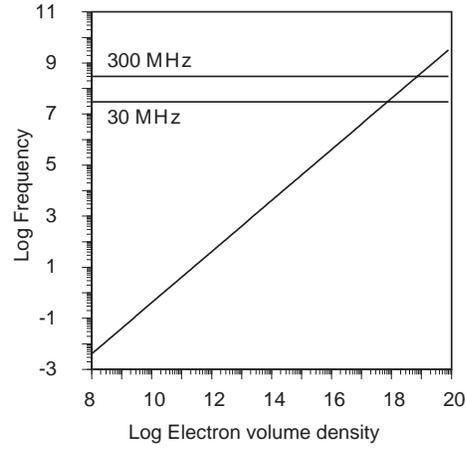
**Fig. 3.** Electron–potassium ions collision frequency as a function of electron density. Temperature 3000 K. Typical radar frequencies are also shown for comparison.
