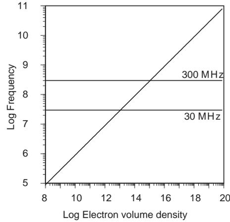
**Fig. 1.** Plasma frequency as a function of electron volume density. Typical radar frequencies are also shown for comparison. SI units are used.
