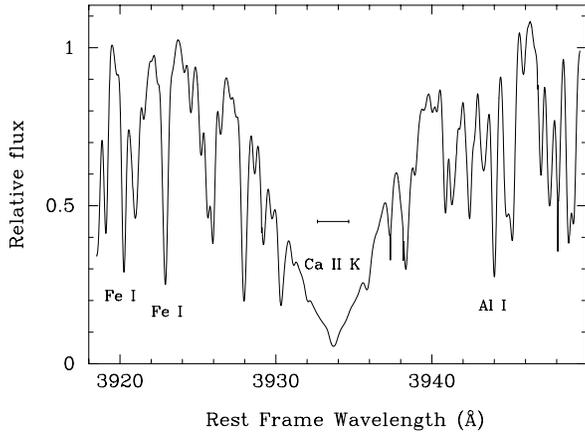
**Fig. 1.** Averaged spectrum taken over one pulsation period. Indicated are the Ca II K line, the two Fe I lines and the Al I line. The horizontal bar shows the domain covered in Figs. 3 and 4
