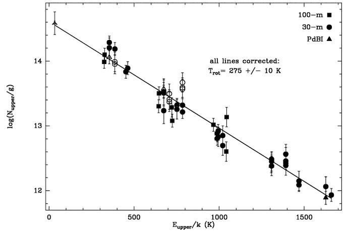
**Fig. 12.** Boltzmann plot of all vibrationally excited HC<sub>3</sub>N lines corrected for optical depth (without taking line broadening into account) with a source size of 0.95'', an isotopomeric ratio of 40, and a line width of 8 km s<sup>-1</sup>. Different Symbols are used for different telescopes. Filled markers denote lines from the main isotopomer, whereas empty markers denote lines from the <sup>13</sup>C and <sup>15</sup>N substituted isotopomer.
