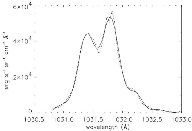
**Fig. 4.** Optimal filter (solid line) applied to an O VI 1032 Å raw profile (dashed line) located in  $(X,Y) = (639,-178)$  arc sec. Frame 07:28:55 UT in Fig. 7.
