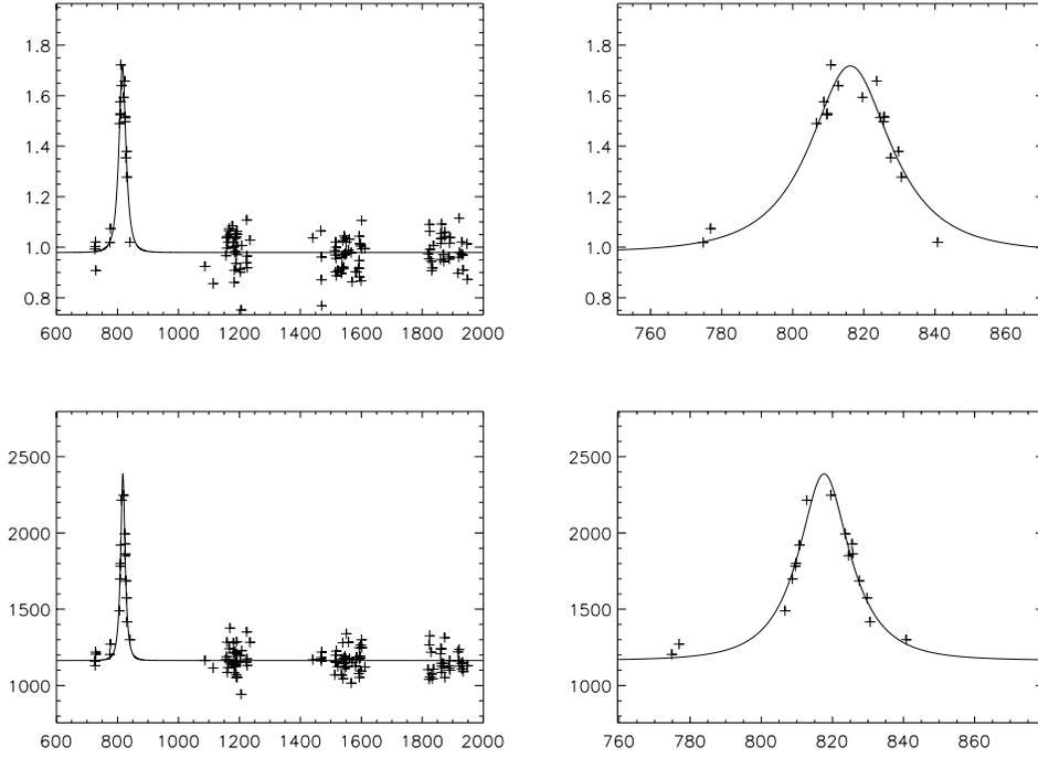
**Fig. 8.** OGLE #9 light curves. The *upper* light curves were obtained with DoPHOT, the *lower* with the image subtraction method. Note a completely different shape of the light curve obtained with image subtraction. This example shows that large biases can be present in the DoPHOT processed data. Image subtraction not only improves the photometric accuracy, but it also eliminates most biases.
