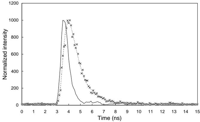
**Fig. 1.** Lifetimes were measured using the method of laser induced fluorescence. The solid line shows the recorded pulse and the dashed line the fitted fluorescence decay curve. The data points for the fluorescence are marked as x in the figure. The curve was recorded observing the decay from the upper level  $v^2D_{3/2}$ , and the lifetime was found to be 770(80)ps.
