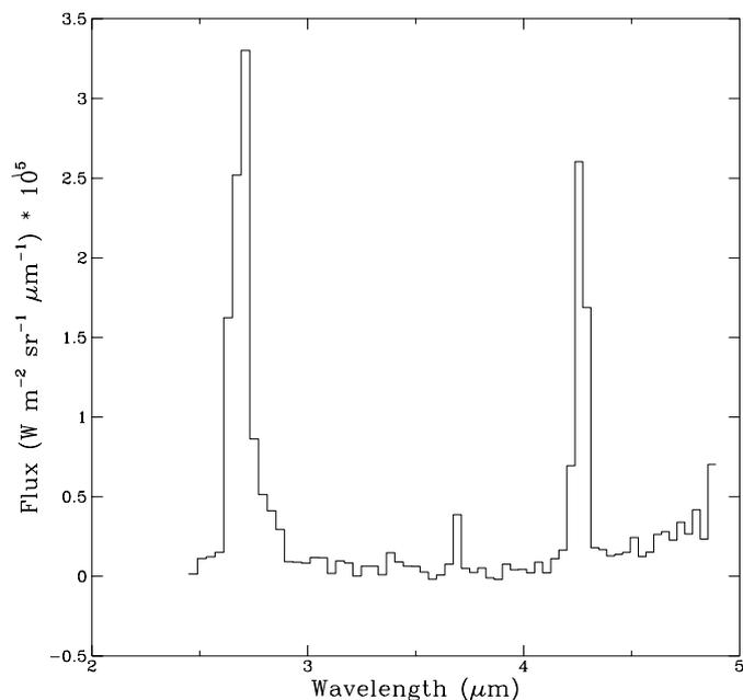
**Fig. 1.** The 2.5–5  $\mu\text{m}$  spectrum of comet 103P/Hartley 2 obtained with ISOPHOT-S on 1 January 1998. The percent errors on the band peak intensity are of the order of 20%
