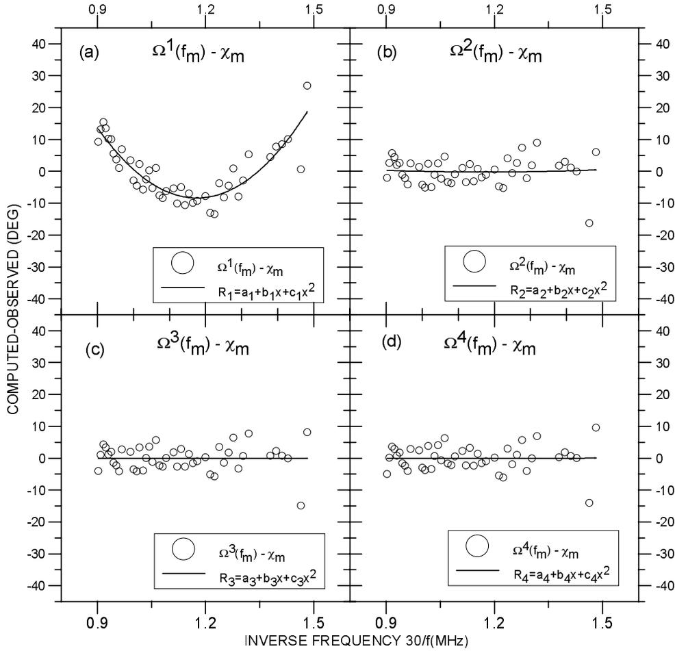
**Fig. 4a–d.** Residuals after the fit of different types of FR models for the spectral cut.  $R_i$  is the fitting curve and  $x = 1/f$ .
