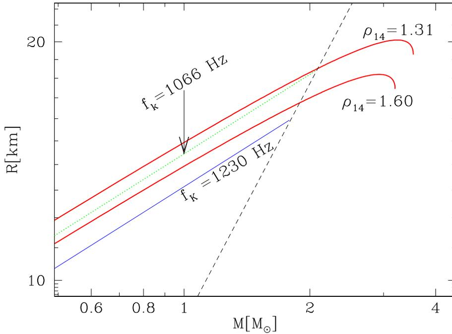
**Fig. 2.** If 1066 Hz is an orbital frequency just above the surface of a strange star, the mass–radius curves of the star (modeled with the e.o.s. [1]) must lie between the two thick curves labelled “ $\rho_{14} = 1.31$ ” and “ $\rho_{14} = 1.60$ .” A circular orbit of frequency 1230 Hz would then never be outside the stellar surface, as it would have a smaller radius (straight line segment labelled “ $f_k = 1230$  Hz”). The dashed line indicates the radius of the marginally stable orbit.
