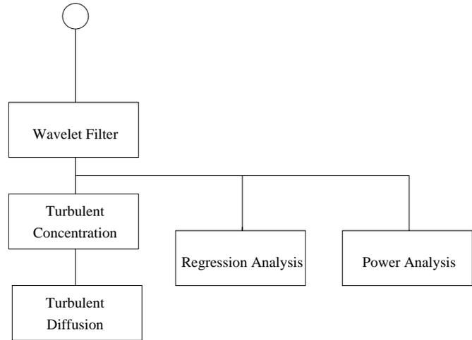
**Fig. 1.** Flow chart of the data processing steps
