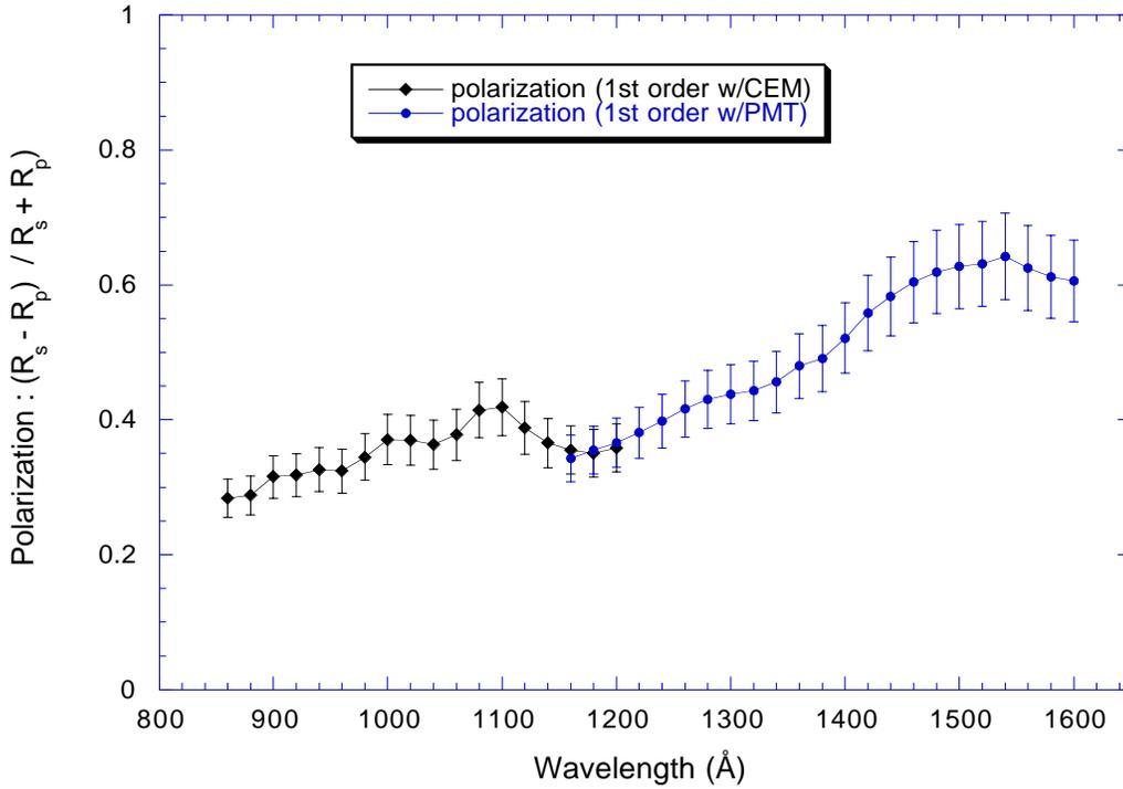
**Fig. 2.** Summary of the measured polarization sensitivity (modulation) of the SUMER instrument from 800 to 1600 Å.  $R_s$  and  $R_p$  are the intensities of the reflected radiation (by the wavelength scan mirror and the holographic grating) respectively parallel and perpendicular to the direction of polarization of the incident beam. Error bars represent roughly one sigma (68%) confidence level in the measured values (taken from Hassler et al., 1997, Fig. 6.)
