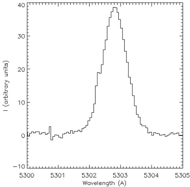
**Fig. 4.** An example of the Fe XIV 5303 Å line from the Norikura coronagraph. The width of the line is 0.8 Å, with the Doppler shift of  $-3 \text{ km s}^{-1}$ .
