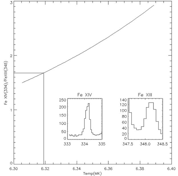
**Fig. 3.** The intensity ratio (Fe XIV/Fe XIII) used to determine the temperature. Sample spectra are shown – the ratio deduced from these particular lines is 1.68 giving a temperature of 2.1 MK.
