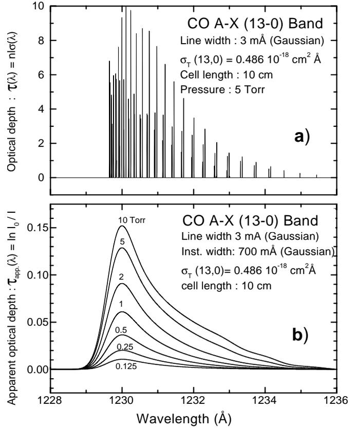
**Fig. 1a and b.** Simulated absorption spectra of the A-X (13-0) band **a** Intrinsic absorption spectrum. **b** Convolution of the intrinsic band absorption spectrum with the instrumental profile.
