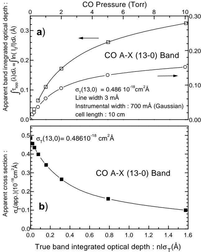
**Fig. 2a and b.** Simulation of the instrumental saturation effects on the A-X (13-0) band **a** Apparent vs. true band integrated optical depth. **b** Variation of the apparent band integrated cross section with true optical depth.
