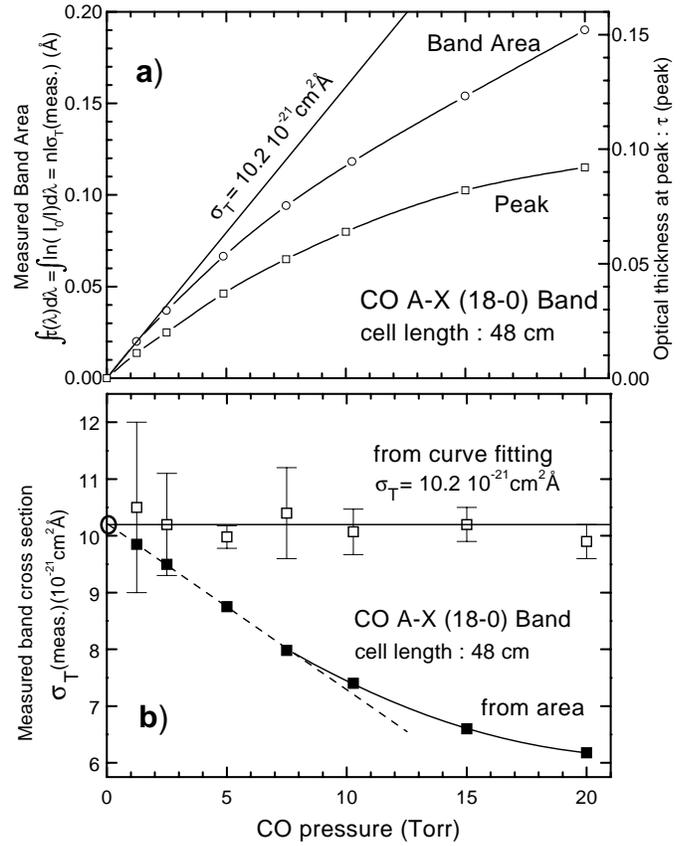
**Fig. 5a and b.** Pressure dependence of the 18-0 band measurements. **a** Band area and peak absorption **b** Cross sections measured through the subtended area and by the simulation/fitting technique
