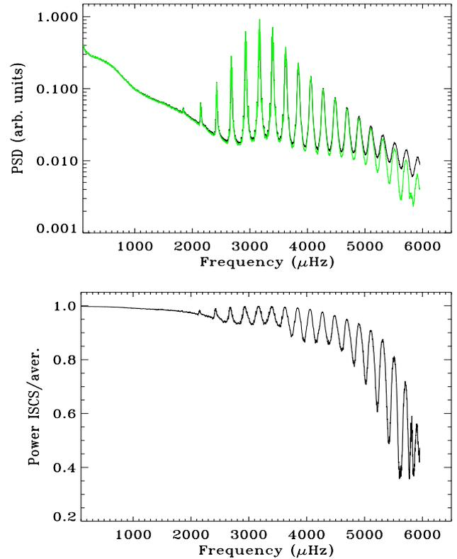
**Fig. 2.** *Top:* The rotation corrected spectrum for  $\ell = 100$ , computed from 61.8 days of full-disk Ca II K-line intensity images. Average power spectrum, AVER (black line), and the ISCS (gray line). *Bottom:* The ratio ISCS / AVER. The improvement in the peak-to-background ratio for the ISCS is readily visible above 2 mHz.
