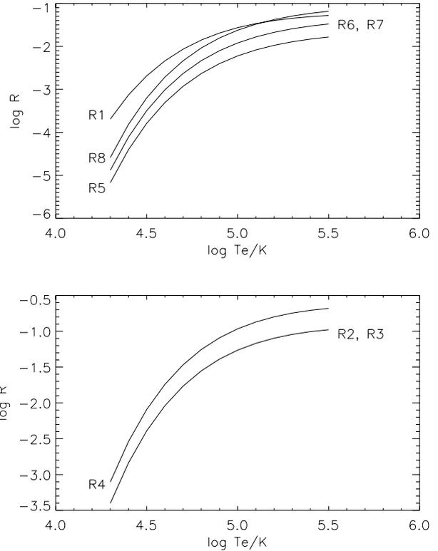
**Fig. 2.** Theoretical Si IV line intensity ratios  $R_1$  to  $R_8$ , plotted as a function of electron temperature. We note that  $R_2$  and  $R_6$  are indistinguishable from  $R_3$  and  $R_7$  respectively, so only one ratio is plotted in each of these instances.
