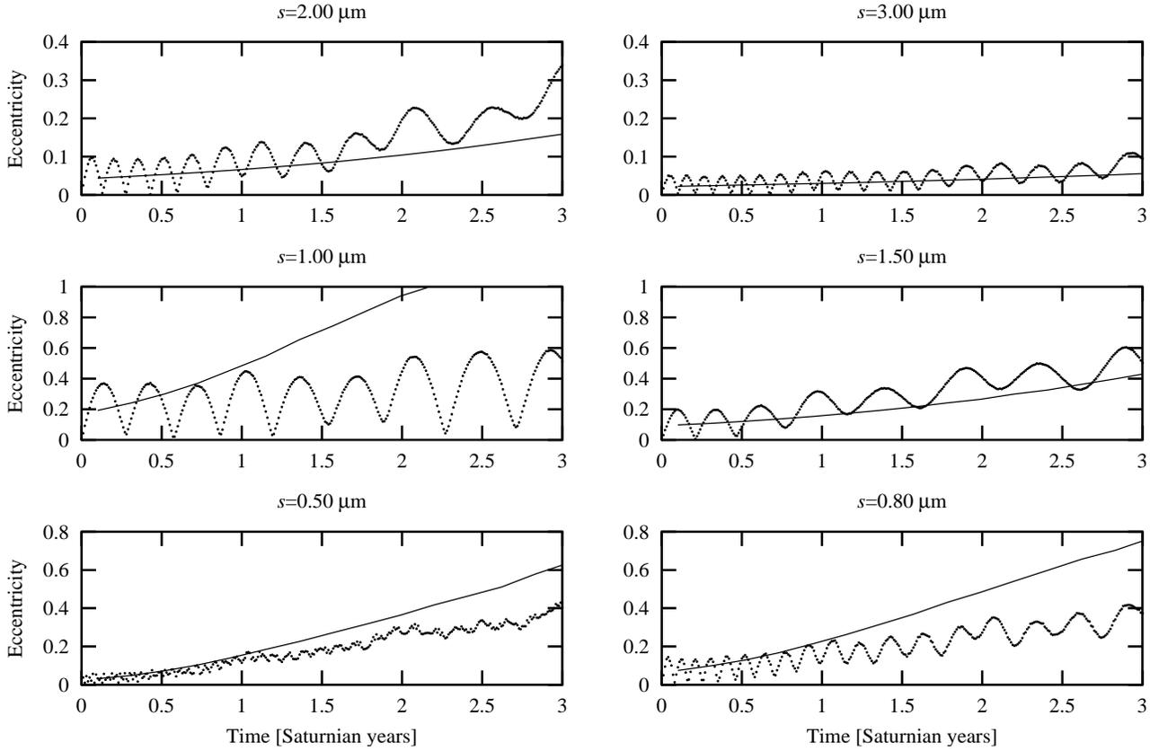
**Fig. 5.** The evolution of eccentricity ( $e = \sqrt{h^2 + k^2}$ ) for different-sized grains with the constant charge of  $-5.6$  V (dots). Solid line shows  $|C\gamma^{-1}|$ . Time is measured in Saturnian years.
