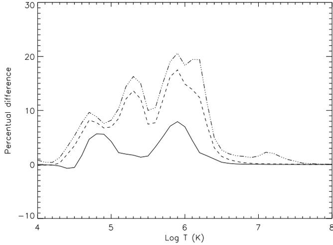
**Fig. 5.** Percentual differences between total emissivity curves calculated assuming different values of the electron density. *Full line:*  $10^8$  vs.  $10^{10} \text{ cm}^{-3}$ ; *Dashed line:*  $10^8$  vs.  $10^{12} \text{ cm}^{-3}$ ; *Dash-dotted line:*  $10^8$  vs.  $10^{14} \text{ cm}^{-3}$ .
