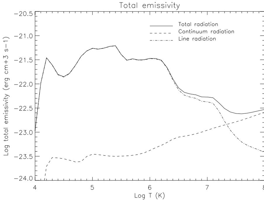
**Fig. 1.** Total radiated power per unit  $N_e^2 dV$  as a function of electron temperature, calculated at  $N_e = 10^{10} \text{ cm}^{-3}$ .
