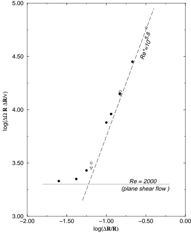
**Fig. 1.** Critical Reynolds number vs. aspect ratio; filled circles from Taylor (1936), open circles from Wendt (1933). Dotted line: critical Reynolds number for plane shear flow instability; dashed line: critical gradient Reynolds  $Re^*$  for circular shear flow in the limit of large gap (see text).
