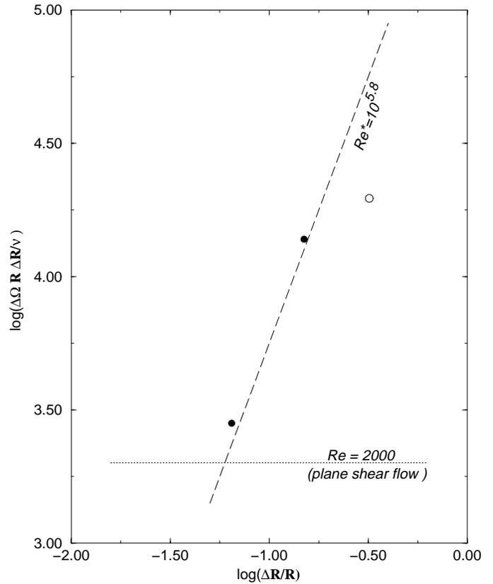
**Fig. 4.** Reynolds number vs. aspect ratio for the three “neutral” experiments from Wendt: the two filled circles correspond to the unstable flows, the open circle to the stable flow. The stability curve obtained for the inner cylinder at rest (Fig. 1) is displayed for comparison.
