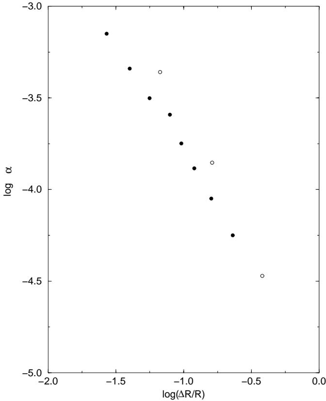
**Fig. 2.** Value of parameter  $\alpha$  in the classical viscosity prescription  $\nu_t = \alpha R \Delta\Omega \Delta R$ , derived from Taylor (1936) in filled circles and from Wendt (1933) in open circles.
