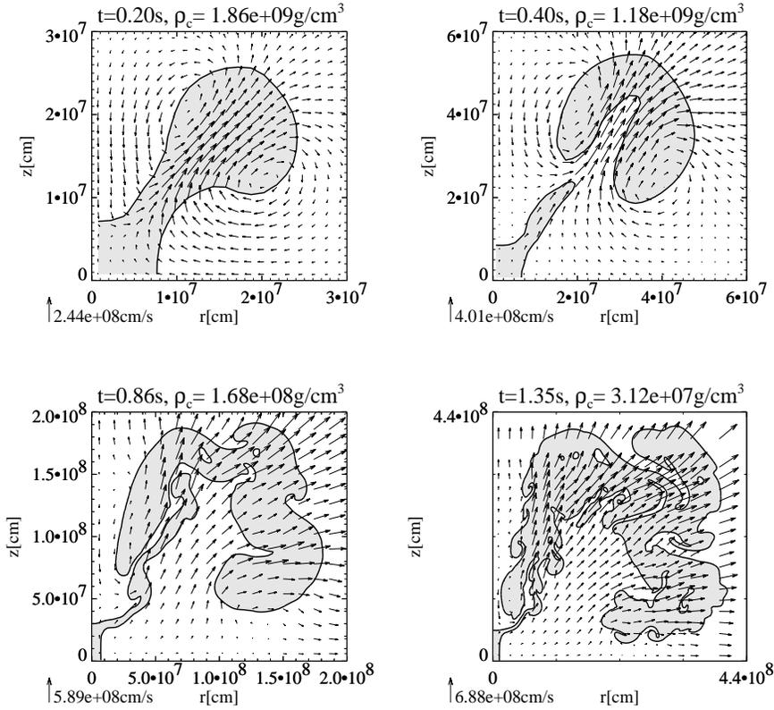
**Fig. 2.** Temporal evolution of front geometry and velocity distribution for model C1. The unequal spacing of the velocity arrows in the last snapshot results from the non-equidistant grid points. Note that all scales change from snapshot to snapshot.
