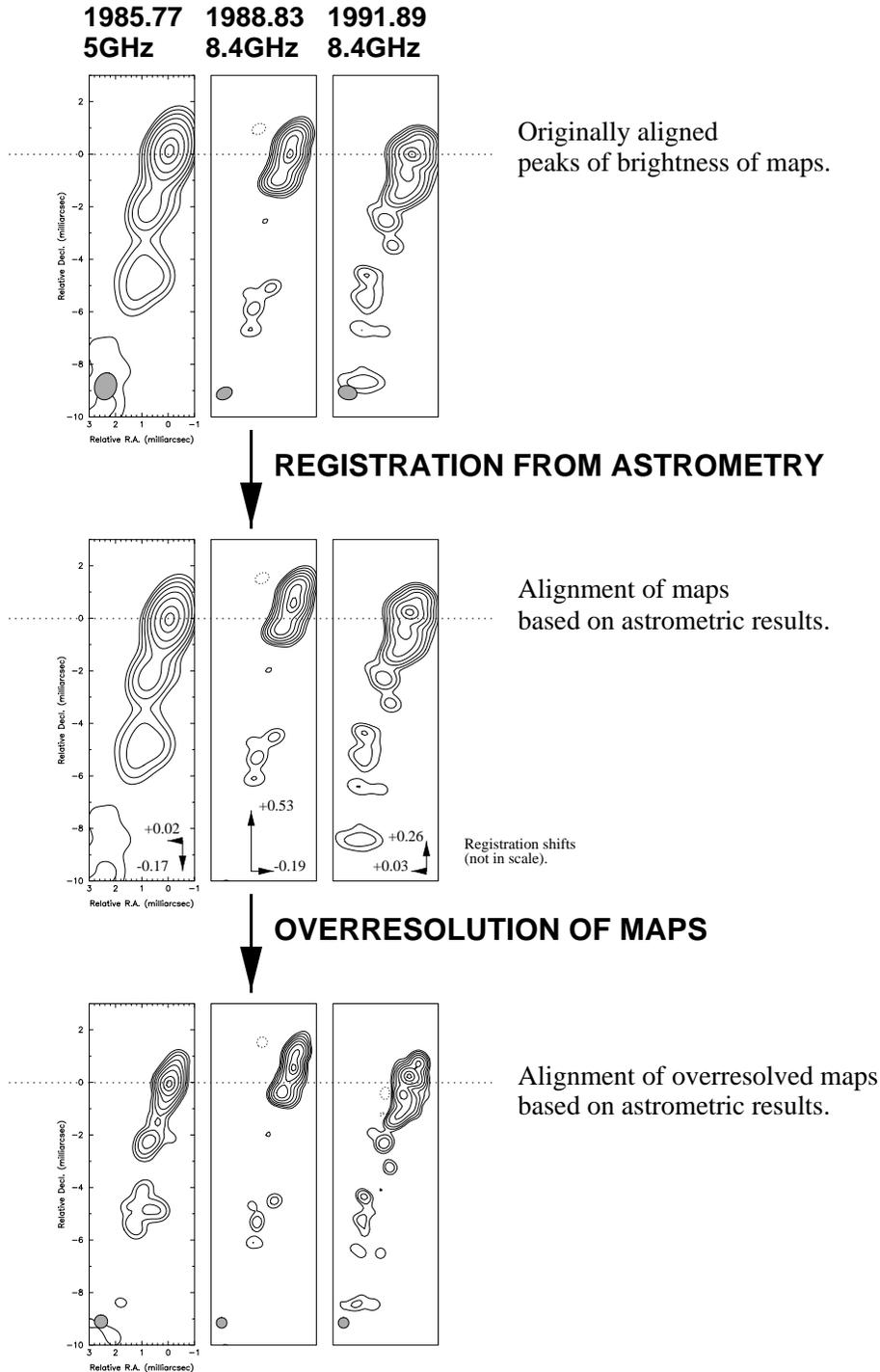
**Fig. 7.** Illustration of steps followed to try to properly align the maps. The astrometric shifts in milliarcseconds are represented (not to scale) at the bottom of the middle figures. The horizontal dotted line in the middle figures passes through the new map origin. The astrometric shifts are the displacements from the origins originally chosen for the maps (upper figures) to the new origins derived from astrometry (see Table 5).
