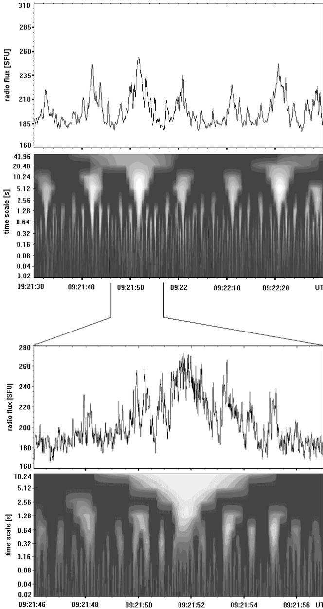
**Fig. 5.** Radio flux time profile at 3 GHz of the event No. 9 of February 16, 1992 (Ondřejov) and the corresponding scalogram (upper part) and a blown-up detail of the same (lower part). The white patterns represent the dominant time scales.
