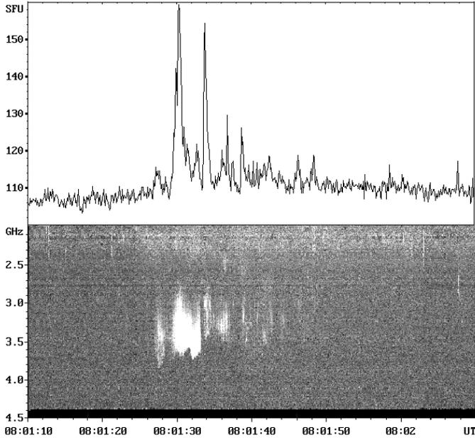
**Fig. 2.** An example of the type 41 F burst at 3 GHz and the corresponding 2.0 - 4.5 GHz radio spectrum (observed on April 15, 1998 at Ondřejov)
