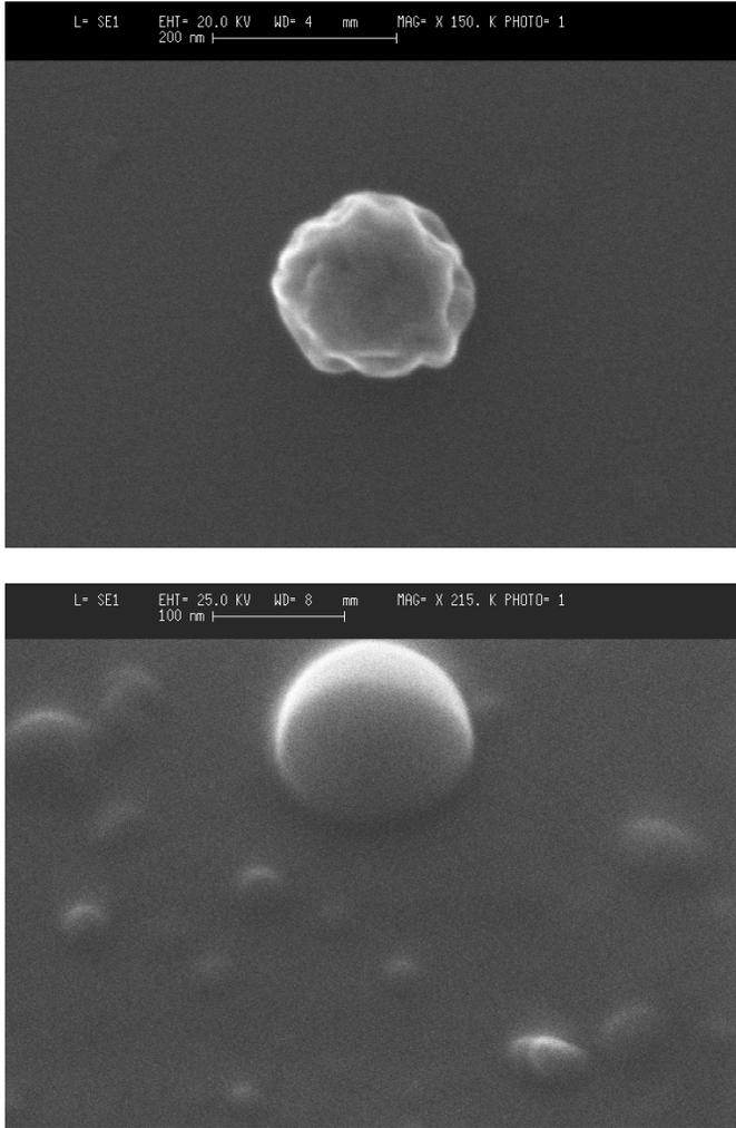
**Fig. 6.** FESEM images of amorphous enstatite produced by laser evaporation (*bottom figure*) and after annealing at 1000 °C for 7<sup>m</sup> (*top figure*).
