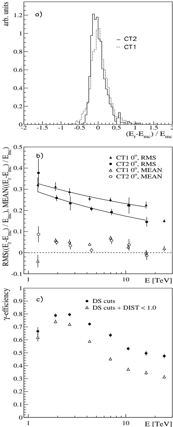
**Fig. 2.** **a** Comparison between MC input energy and reconstructed energy. For the energy spectrum a power law with a differential coefficient  $-2.2$  is assumed; **b** Predicted energy resolution as a function of  $\gamma$  energy and relative deviation between the mean reconstructed energy and the initial energy. For CT1 and CT2. **c** Overall cut-efficiencies for standard cuts (DS) and for harder cuts used for the spectrum analysis.
