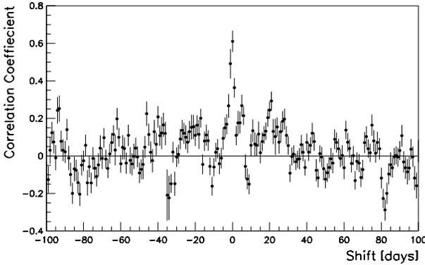
**Fig. 10.** Check of the correlation between the X-ray emission of Mkn 501 in 1997 as measured by RXTE and the emission above 1.5 TeV as measured by CT1. Plotted is the correlation coefficient as a function of the artificially introduced shift between the RXTE and the CT1 time.
