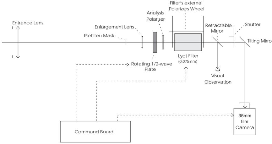
**Fig. 1.** Schematic representation of the H $\alpha$  polarimeter in Meudon
