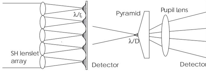
**Fig. 1.** The SH (left) and the pyramidic (right) WFS compared; both the WFS are shown in the perfectly close loop situation. When a tilt of the order of  $\lambda/D$  is introduced the efficiency of the pyramidic WFS is much larger because it acts *after* the recombination of the whole pupil light. In fact the movement of the spot is comparable to its size, while in the SH case all the spots will move of a fraction of their size.
