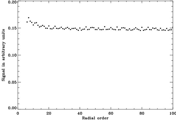
**Fig. 2.** In this plot the returning normalized Peak to Valley signal is given with respect to a Zernike polynomial wavefront of  $\lambda/20$  Peak to Valley. Sampling of the pupil is made with a  $128 \times 128$  array.
