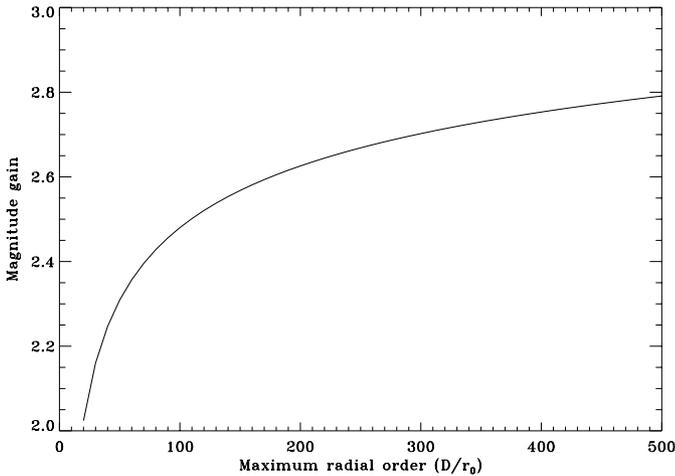
**Fig. 4.** The gain in limiting magnitude for different  $Q = D/r_0$  cases.
