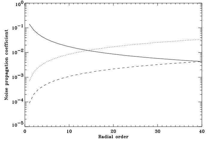
**Fig. 3.** Solid line:  $p_i$  vs. the radial order  $q$  for the SH case; dotted line: the same for the pyramidal case; dashed line: the same scaled in order to have the same integral area for the WF residual error.
