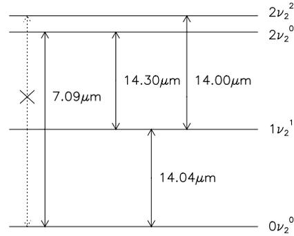
**Fig. 5.** The energy levels of HCN and the wavelengths of transitions in the  $\nu_2$  bands
