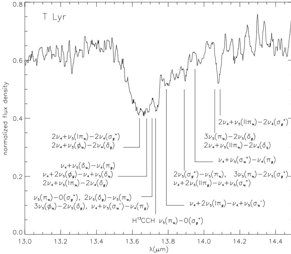
**Fig. 7.** The normalized spectrum of T Lyr with the identification of the  $Q$  branches of the  $C_2H_2$   $\nu_5$  bands, including that of the  $H^{12}C^{13}CH$   $\nu_5^1$  band
