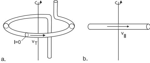
**Fig. A1.** **a** Rigid ring-shaped tube segment rotating around the ring axis. **b** Tube rotating around a minor axis with internal flow.
