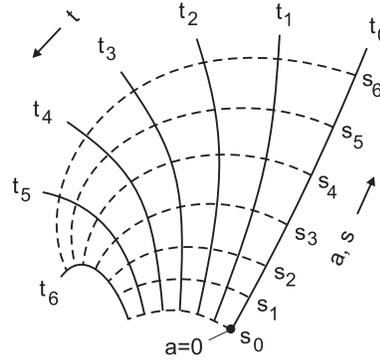
**Fig. 1.** Thin magnetic tube at time  $t_0$  and at a later times  $t_1, \dots, t_6$ . The lines  $s_i = \text{const}$ ,  $i = 0, \dots, 6$ , are orthogonal to the momentary tube axis.
