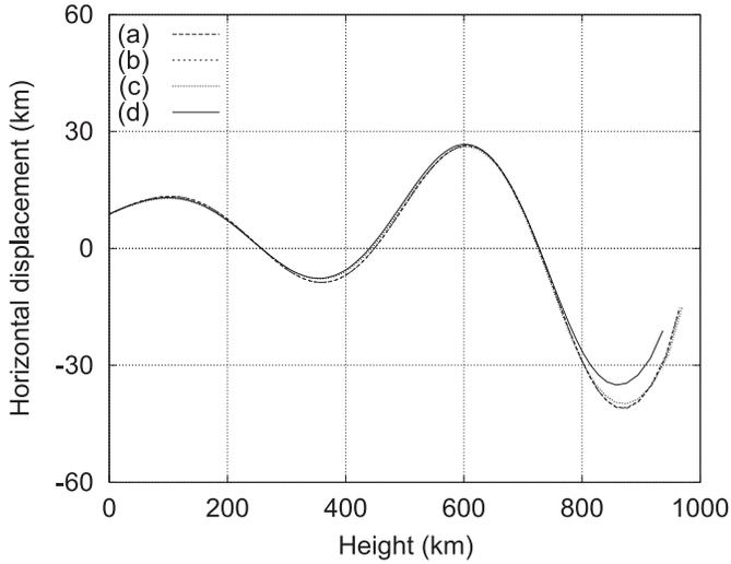
**Fig. 2.** Horizontal displacement  $x$  versus height  $z$  of the magnetic flux tube axis for a longitudinal-transverse wave with period 90 s, 600 s after the start of the sinusoidal shaking at the bottom. Curves are labelled according to Eq. (48). The curve labeled ‘(a)’ reproduces a calculation of Paper I.
