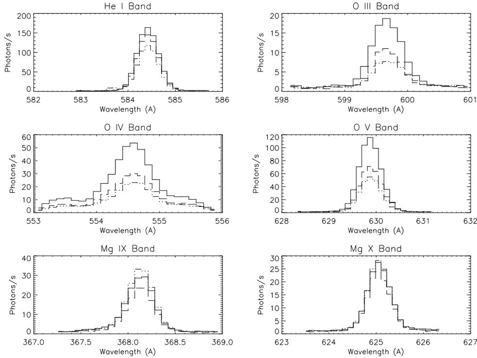
**Fig. 2.** The six wavelength bands used in the blinker analysis, centred on the lines He I 584 Å, O III 599 Å, O IV 554 Å, O V 629 Å, Mg IX 368 Å, Mg X 625 Å. Three curves are shown for each, for the pre-event (dashed), event (solid) and post-event (dash-dot) phase for a blinker on 4 December 1997. This is a 75 raster run (Table 2), and the spectra are taken from a sum of the 5x5 pixels for the rastered images 20, 27 and 41.
