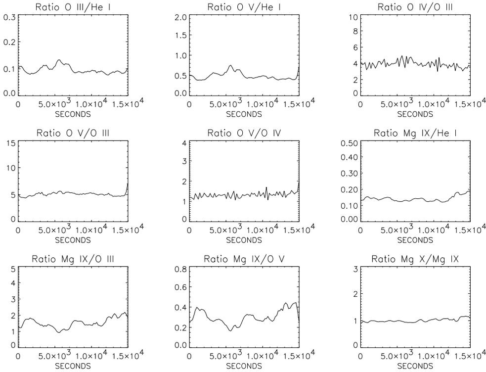
**Fig. 4.** For the same period and pixel group used in Fig. 3, the ratios of the intensities of the various emission lines are plotted. The behaviour of these ratios can be used to determine temperature and density variations.
