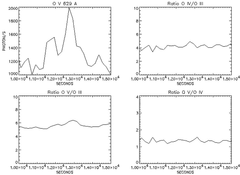
**Fig. 9.** A blinker recorded on 22 November 1997 in O V. The intensity of the O V line plotted against time from the start of the observation run is shown in the top left panel. For the same time period, the remaining three panels show the ratios of the O IV/III, O V/O III and O V/O IV intensities. No significant increases or decreases are detected during the blinker event.
